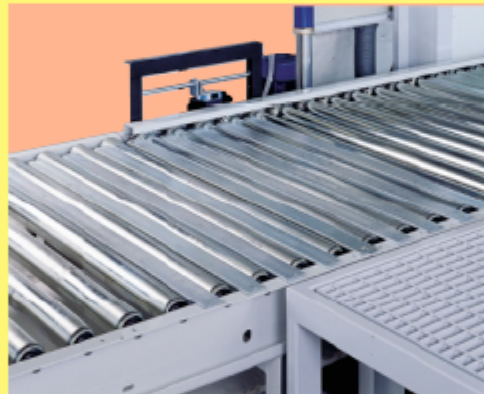
Roller conveyor (with operator access).
