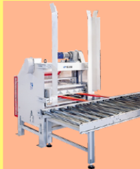
Magazine with retractable forks.
